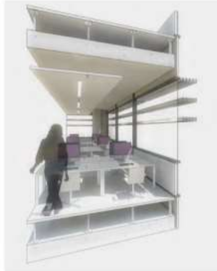
Base Design - External Brise Soleil
