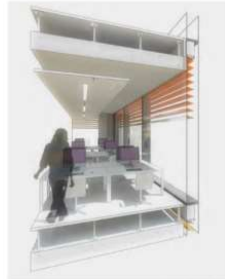
Closed Cavity Facade
